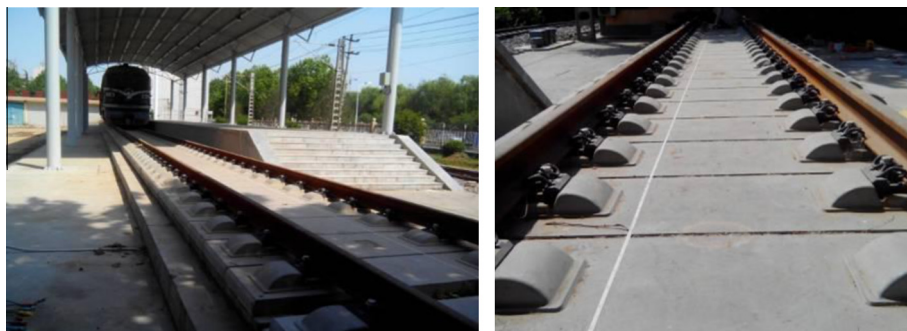
Fig. 14. Real model of ballastless high-speed railway undertrack structure.
